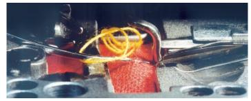
NEEDLE POINT HAS ENTERED FABRIC. SPLIT-OFF FIBRES ARE SHIFTED UP ON THE POINT CONE.
