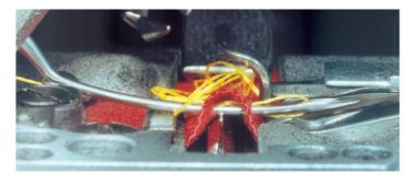
NEEDLE JUST BEFORE PENETRATION. THE BALL POINT HAS IMPEDED THE SEPARATION OF FIBRES FROM THE CLOTH AS IT CAUSED THE NEEDLE TO DEFLECT. A SKIPPED STITCH IS THE CONSEQUENCE .
